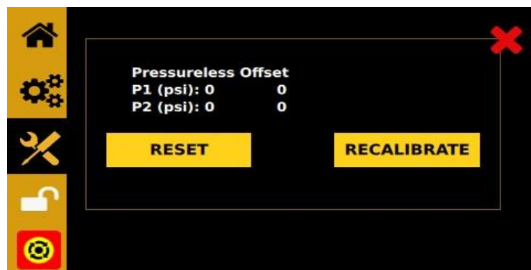
Figure 14: External Pressure Calibration Screen
