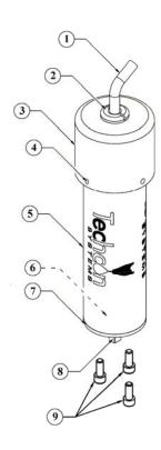
NOTE: When replacing the motor (6) and square drive (8), Loctite #86 AVV must be used, to bond the square drive to the motor shaft. The square drive must be flush with the end of the motor shaft and any visible excess must be cleaned off.
