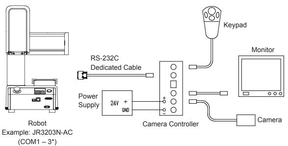
\* Do not set the start channel to the same COM port that the camera is connected to. A camera communication error will occur.
