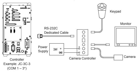
\* Do not set the start channel to the same COM port that the camera is connected to. A camera communication error will occur.
