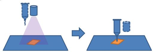
So long as the workpiece is within the camera shooting range, it can be placed freely
