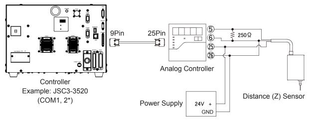
\* To use COM1 to communicate with a distance sensor, set COM1 Command Communication Function to Invaild. The following procedures are necessary for using this function.
