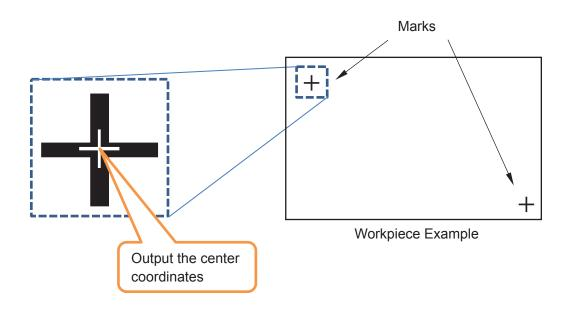
Calibration Mark Coordinate Output Settings (ASCII text settings)
