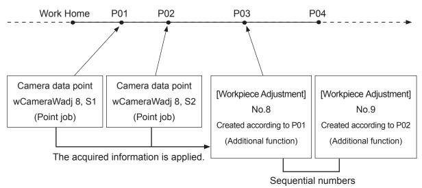
Camera data acquisition is performed at P01 and P02. This information is applied to the additional function [Workpiece Adjustment] set at P03, thereby finalizing P03's position (P03 coordinate values + adjustment values).
