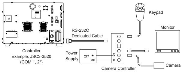
\* To use COM1 to communicate with a camera, set COM1 Command Communication Function to Invaild.
