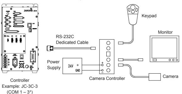
\* To use COM1 to communicate with a camera, set COM1 Command Communication Function to Invaild.
