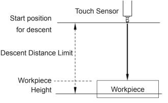
specified in [Distance Limit] and the touch sensor does not come ON, an error occurs.
