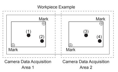
If you create a calibrated workpiece adjustment to match point (1) (camera data acquisition point (1)) and set it to both points (2) and (4), the workpiece adjustment set to point 4 deviates from the correct position. The reason for this deviation is in the workpiece adjustment calculation method.
