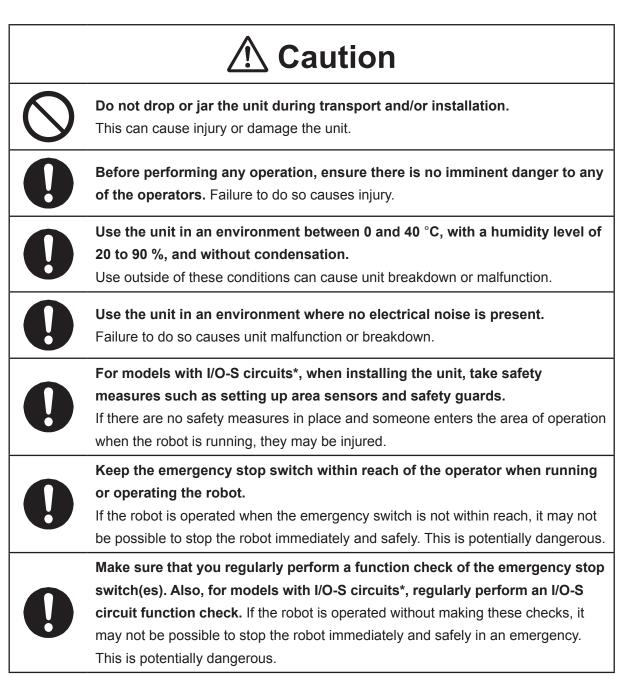
\* A stop made via a device connected to the I/O-S connector is a category 2 stop. Make sure to perform a separate risk assessment of the interlock device.
