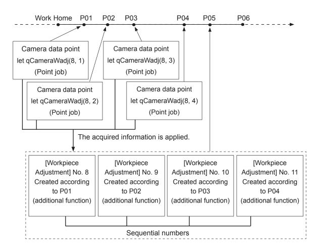
Camera data acquisition is performed at P01, P02, P03 and P04. This information is applied to the additional function [Workpiece Adjustment] set at P05, thereby finalizing P05's position (P05 coordinate values + adjustment values).
