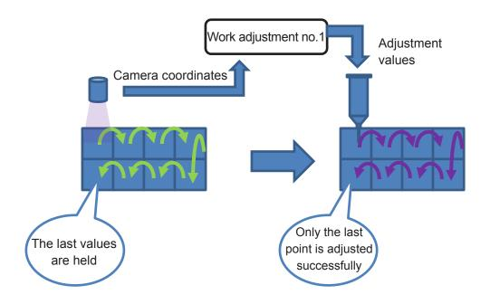
To avoid a situation such as this, you need to handle the workpieces by setting a different workpiece adjustment number to each workpiece for each photograph.
