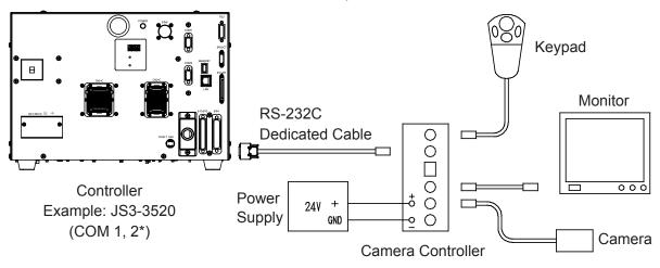
\* Do not set the start channel to the same COM port that the camera is connected to. A camera communication error will occur.
