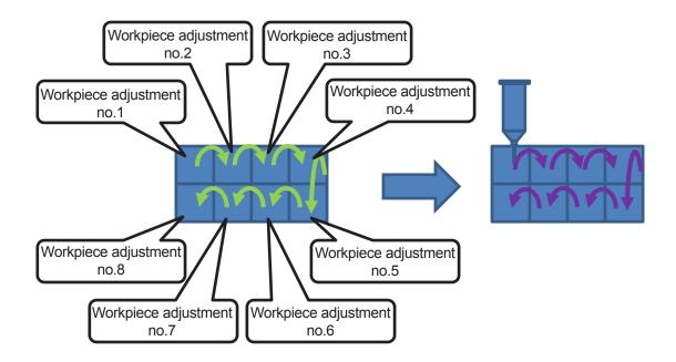
Using this method you can resolve the issue of making workpiece adjustments after first photographing multiple workpieces; however, managing them can be difficult when there are many workpieces.
